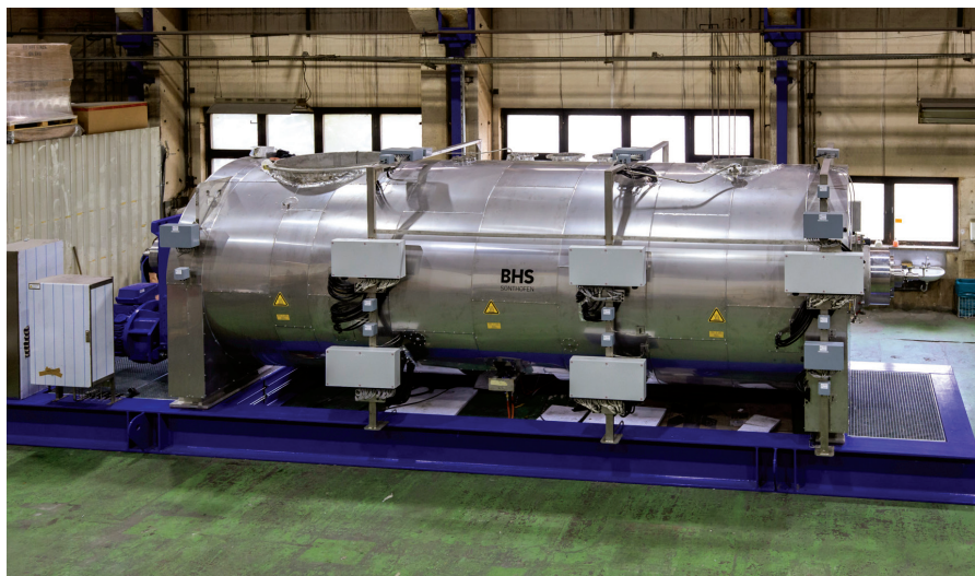
The horizontal dryer makes it possible to work with sticky, viscous materials in pyrolysis applications.
