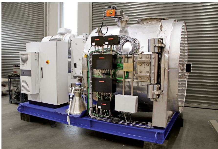
Horizontal dryer used to calcinate minerals. All images courtesy of BHS-Sontheofen.
