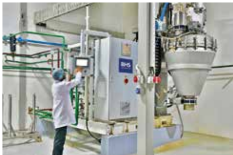
BHS-Sonthofen supplied Granny's Spices with a complete plant including a vertical BHS sterilizer.
